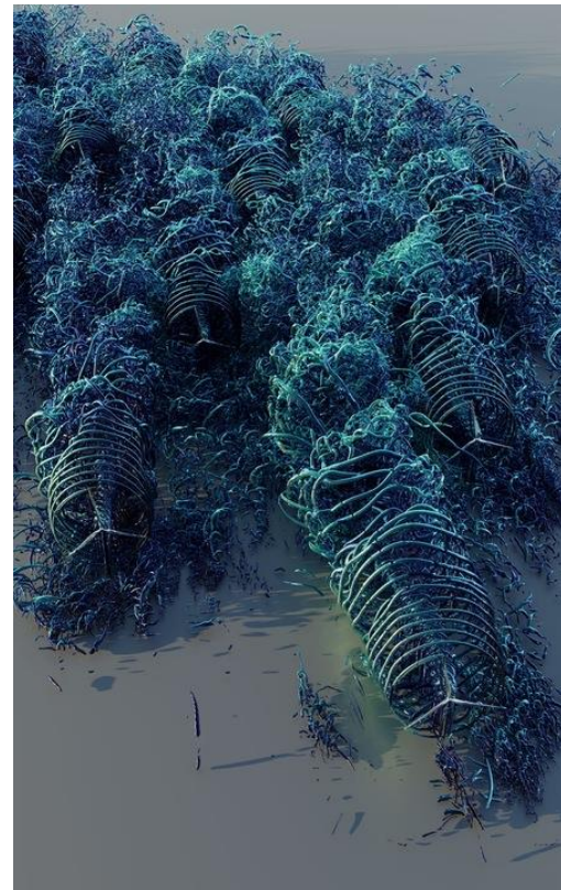
ExaWind hybrid RANS/LES simulation of 16 NREL 5-MW turbines on the Frontier supercomputer; credit Brunhart-Lupo and Cheung
