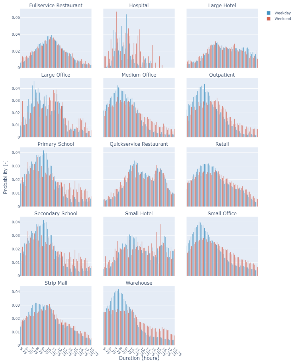
Figure 9. Operating hours' duration distributions.
