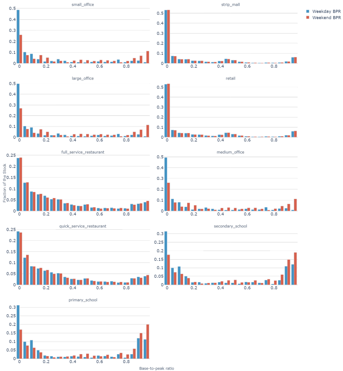
Figure 32. Weekday and weekend lighting base-to-peak ratios by building type. Base-to-peak ratio is on the x-axis, and fraction of the stock is on the y-axis.
